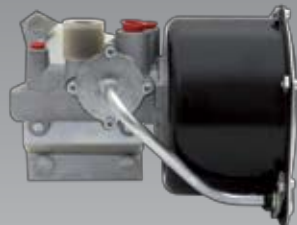
GIRLING POWERSTOP BOOSTERS ARE FITTED TO MANY EARLY ENGLISH & AUST MODELS
